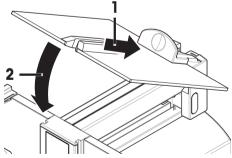
Insert the liquid kit (1), pull 2 levers (2) towards you and slide liquid kit onto the rack.
