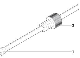
12 To fasten sealing ring, tightly screw fastening nut.
