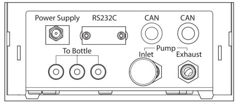
Power supply and RS232C-connector are covered with a faceplate. Remove faceplate.
