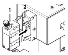
1 Insert liquid dosing head in the liquid dosing head support.
